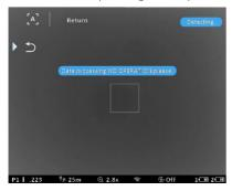
Step 5: When message "Confirm the current options?" user can see a small white cross in the square. If the cross overlaps the heat signature of the projectile impact on the target face, it tells a successful auto zeroing. Click Yes. This confirms that the computer has correctly identified your projectile impact and that the Auto zero process is now complete.
