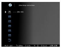
Default value is 0, no correction to the reticle. Select distance. it will enter into the menu below. The message on the left corner tells the value in cm/inch for each one click.
